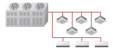
Larger, centralised heat pumps are also available, where a single outdoor heat exchanger is used to heat a large number of indoor units or ducted air supply. The warmed air is then distributed around a building via these ducts and enters the individual rooms via vents.
