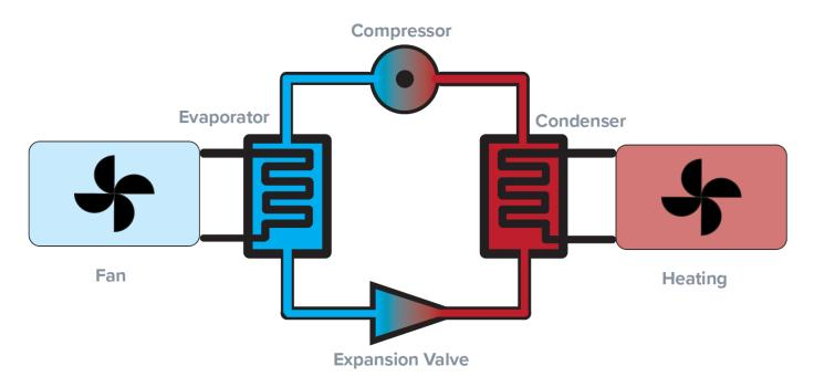
The evaporator is located outside and is a large, finned heat exchanger which has a fan to drive ambient air over it. The compressor consumes electricity to raise the temperature and pressure of the refrigerant gas in the system. The condenser is a heat exchanger which gives up the heat to the building or hot water system that is to be heated. There are two common types of AtW heat pumps:
